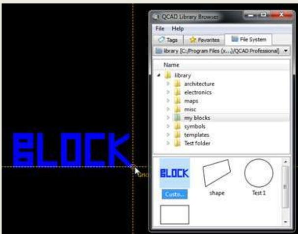
5. When inserting the block (part) will be given the options to rotate or scale the block as well as layer options! See below.
